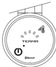
When the set time elapses, the heating element automatically returns to the settings from before the activation of the timer function. With the TIMER function active, you can freely modify the operating temperature (
