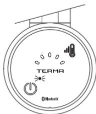
Pairing mode, when activated, lasts 30 seconds.
