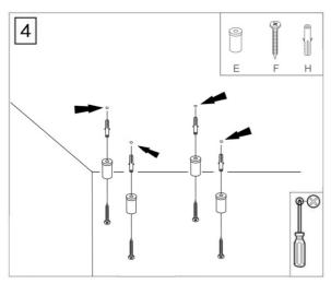
5. Attach ceiling lock screws (D) to suspension wires. Screw (D) tight into (E).
