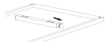
Slide the panel onto the hanging brackets, as per the diagrams below. Slot the mounting bars all the way onto the hanging brackets on one side. Raise the panel until it is level with the ceiling and pull it back so the mounting bars slot onto the other two brackets.
