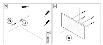
5. Slide the panel across so that the screws lock into their correct position in the bracket, as pictured below:
