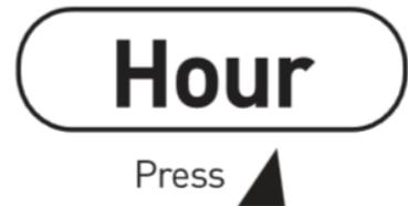
The programmer will then move on to setting the time. The hour will flash to indicate it is selected and can be changed using the up or down arrow buttons. Press OK to confirm the hour and repeat the process with the minutes.
