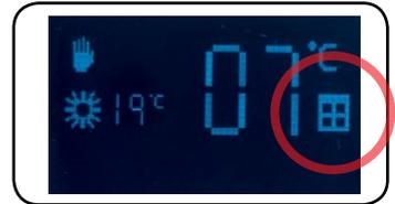
When closing the window, the radiator will detect a temperature rise and this function will be deactivated.
