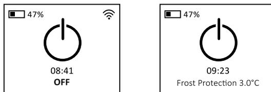
Figure 2 | OFF with frost protection disabled (left), enabled (right)
