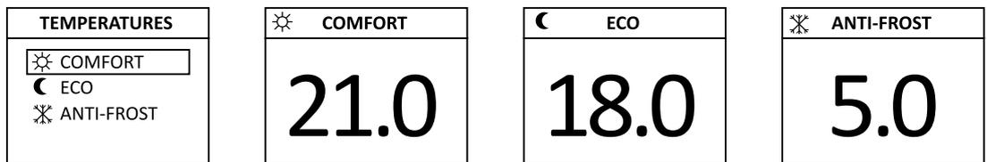
Figure 3 | Preset temperatures: comfort, eco, and anti-frost
